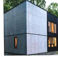
6. NATURAL FINISH FIBRE CEMENT CLADDING
